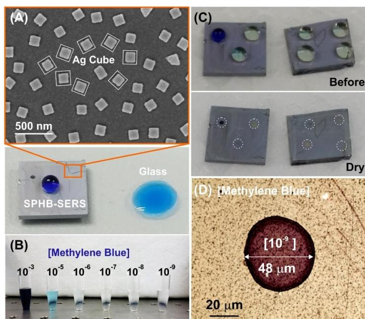
**Figure 1. Characteristics of superhydrophobic-SERS platform.**
