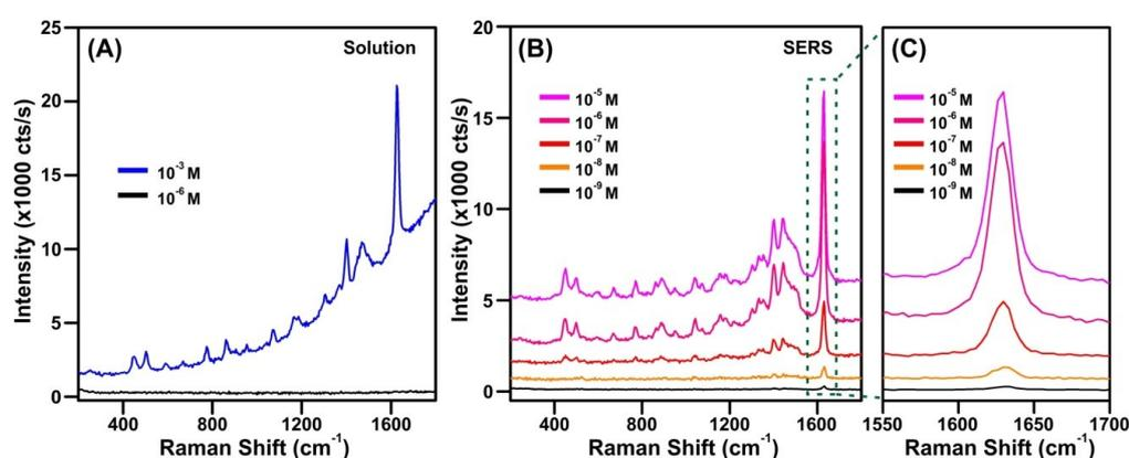
**Figure 2.** Raman spectra collected from (A) MB solutions, and (B) MB deposited on our SPHB-SERS platforms.
